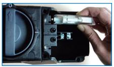
Snap into side(s) of terminal block
